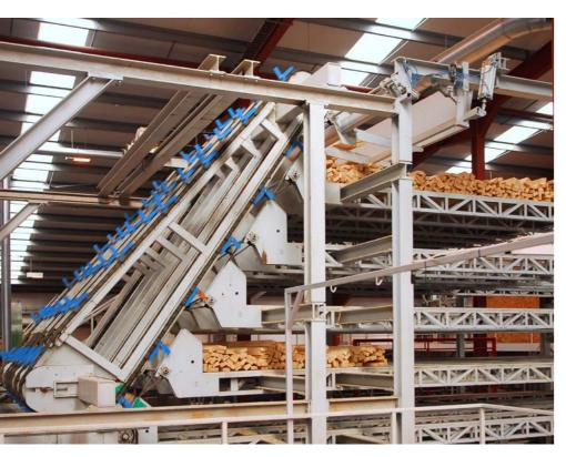
**Buffer layer sorters** loosely sort batch material on top of each other into layers. The material must be separated before filling and after emptying the system.
