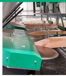
If required, incising units for surface perforation, as preparation for impregnation with wood preservatives, can also be integrated into a post-pointing production line. Even before perforation, lumisensors detect unsuitable wood marked with luminescent chalk. In this case, the unsuitable wood is sorted and discharged through a flap.
