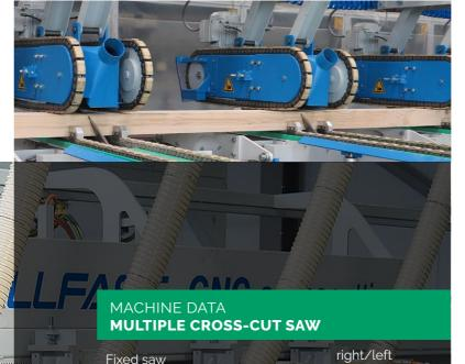
500 mm Min. cutting length 16,000 mm Max. cutting length 200 mm Max. cutting thickness 1 mm Cutting accuracy 5.5 - 18 kW Saw motor output 3 kW Feed capacity 50 m/min Max. feed rate
